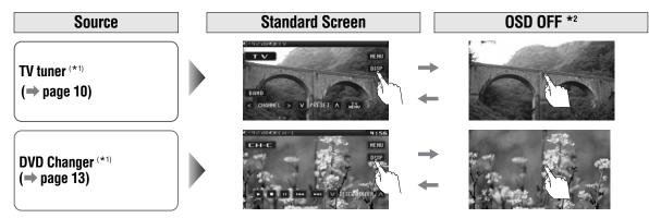
\*1 To switch Operation Screen ON, touch the center of touch panel or press [ENTER] on the remote control.
